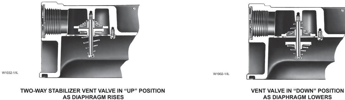
**Figure 5.** Types 133H, 133L, and 133Z Stabilizer Vent
